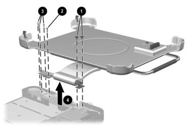
Removing the Docking Stand and Pivot Arm
